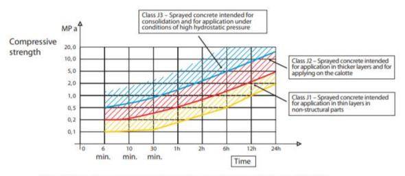
Class of sprayed concrete according to the strength properties in the first 24h
